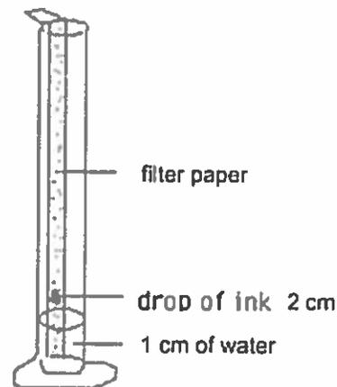
Set up of filter paper and cylinder
