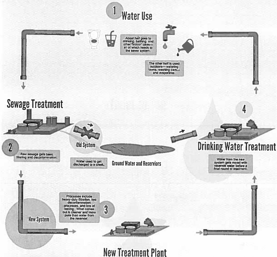
Figure 1. Diagram showing how a direct potable reuse system works in Big Spring, Texas. Taken from marketplace.org
